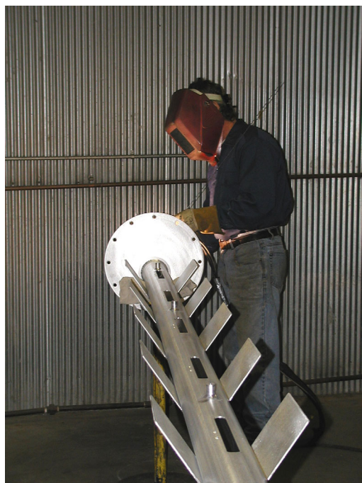
PSILP SLOT ANTENNA IN PRODUCTION AT THE FACTORY.
